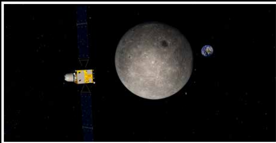
Chang'e-3 was China's first unmanned lunar probe to soft-land on the moon. It incorporated a robotic lander and a lunar rover. The net weight of the probe was 1,220 kilograms, of which the lander was a newly developed spacecraft platform with a weight of 1,080 kilograms and a designed life of 12 months. courtesy of Shenzhou Media
